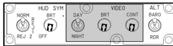
HUD Control Panel FLIR video controls
