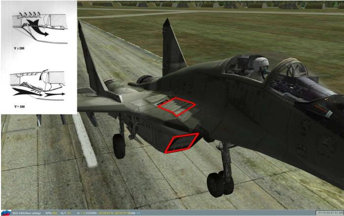
Here, both additional and main air intakes are closed.
