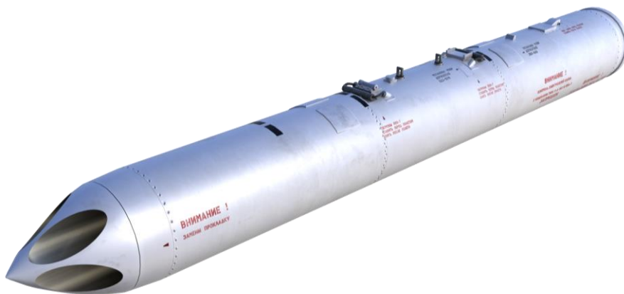
Figure 80 : Lance roquettes UB-13
