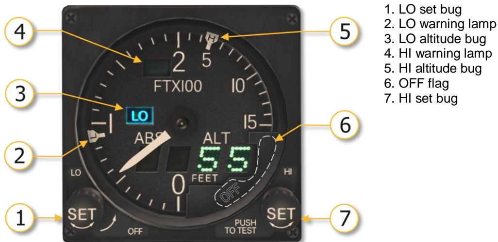
Figure 5.4. AN/APN-209 radar altimeter
