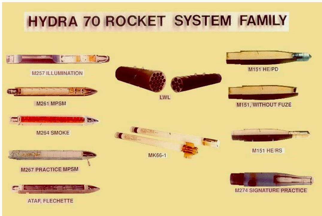
Figure 8.5. 2.75 inch FFAR Warhead Types
