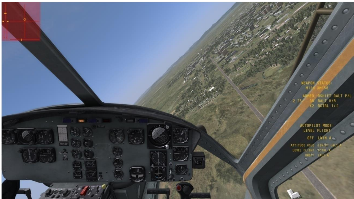
Figure 10.1. Location of the WEAPON STATUS indicators.
