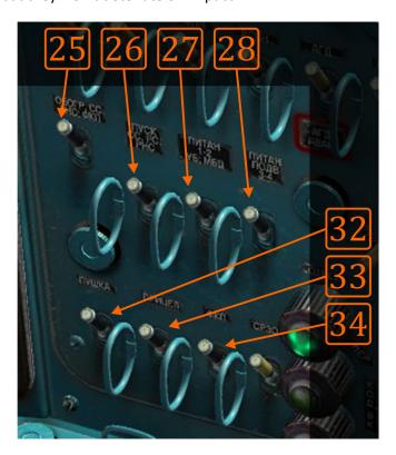
**Image 10.1**: Weapons activation interface on right-vertical panel.
