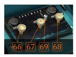
The Flaps Control Panel is used to operate flaps and indirectly indicate flaps position. Button (LV68) retracts the flaps, while buttons (LV67) and (LV66) serve to set the flaps to takeoff (25°) or landing positions (45°), respectively. Button (LV69) serves to set all the control buttons to upward position (to relieve the buttons' springs when aircraft is not in use; no in-game practical use).
