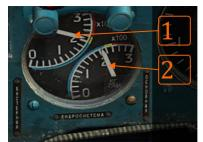
Hydro pressure gauges indicate pressure in both hydro systems: main and command. Main hydro system (2) provides hydraulic pressure for nosecone movements, engine compressor anti-surge door operations, landing gear, flaps, airbrakes, engine nozzle, one hydro-booster chamber of the horizontal tail, tyres breaking action during gears retraction, equipment air-conditioning door operations, and – in the case of command hydro system failure – it
