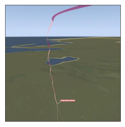
**Image 8.7**: Profile of a flat spin after dynamic entry. On given image, each turn is about 500m altitude loss. If you experience a spin, expect your engine to shutdown. When flying DCS MiG-21BIS always associate spin with high probability of engine shut down. If you manage to recover the plane, you will have to assess whether you have a chance of restarting the engine.
