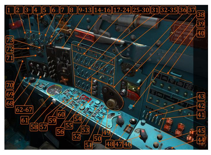
R segment contains interface for turning on/off all the airplane systems. Along with that, RV segment contains main radar control panel, radio station channel selector and ARC station selector.
