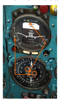
**Image 9.13**: NPP shows the aircraft is within the localizer/glide path radio beams. The presence of the localizer and glide path radio signals is indicated with black windows flashers on NPP (blinker windows, in orange circles). Localizer and glide path needles show the same values both on KPP and NPP (orange arrows).
