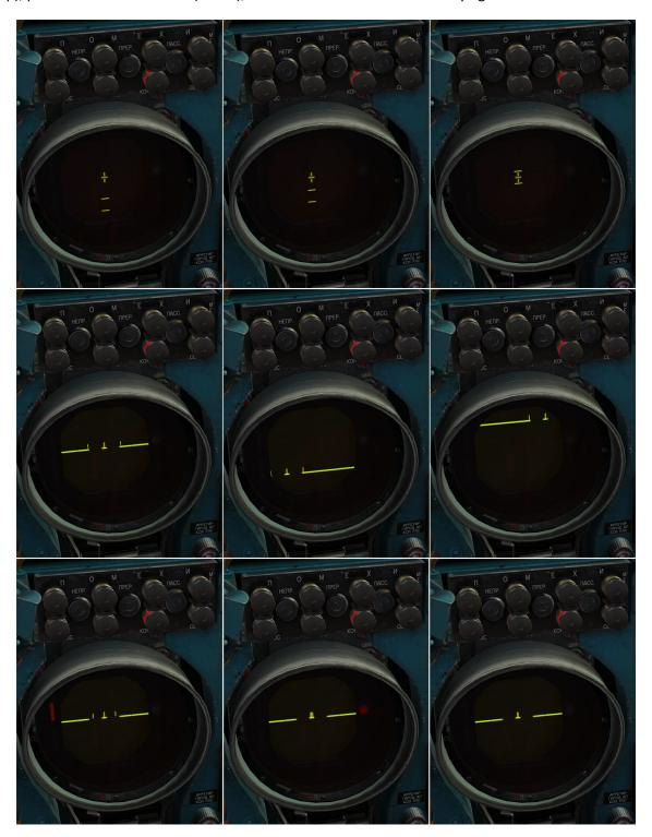
Image 10.7: illustration of radar self-test pattern
