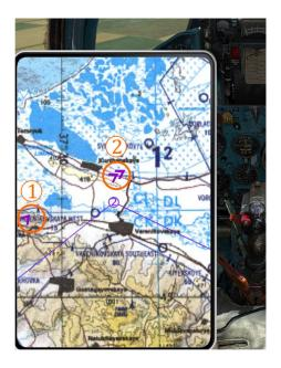
**Image 9.18:** Kneeboard with map of proper scale, flight route and few "position marks". Position mark symbols are violet colored arrow-heads: tip of the arrow-head indicates aircraft direction. Mark 1 was taken several minutes before the screenshot, and it indicates the route is to the right side. I did not correct my trajectory at this point. Few minutes later, I marked two sequential positions (mark 2). Compare positions and the route.
