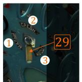
External lights are positional lights and landing/taxi lights. Control switch for positional (AKA formation) lights is located on the right vertical panel (RV29). This switch has four positions: neutral position - lights OFF, position 1 - small intensity lights, position 2 - medium intensity lights, position 3 - maximum intensity lights.
