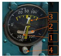
The DA-200, often referred to as the "variometer", will give you precise information about vertical velocity up to 20 m/s, and rough information from 20 m/s to 200 m/s. The Slip ball (2) will indicate slip, while the turn indicator (3) will show you the turn rate. This indicator is specially designed to indicate bank up to 45° in steps of 15° when the airplane is flying at 500 km/h IAS. The purpose of this function is to replace the KPP if it fails, and enable safe landing pattern creation.
