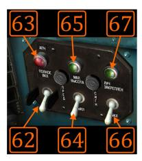
Image 10.6: Main radar control panel.
