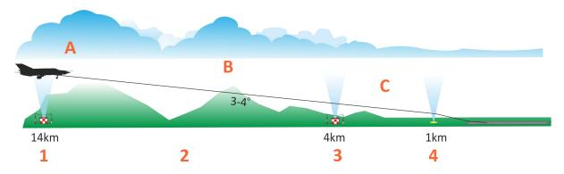
**Image 7.2**: Approach for visual and ARC landing (for ARC landing see Radio navigation chapter).
