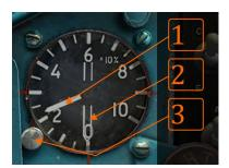
The Nosecone position indicator (UPES-3) shows the current nosecone position in % of maximum extended position (white needle). In case of automatic control system failure, the pilot can switch to manual by using the *Nosecone control switch (LV07)*. A particular nosecone position is set-up by using knob (3) and moving the black-white needle (2) to the appropriate position. As the pilot moves the needle (2), the white needle (1) will follow,
