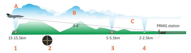
**Image 9.16**: PRMG approach and landing parameters. Picture also shows NDB stations and their distance to PRMG (or RSBN) stations. Note that the above shown NDB locations may not be available for every airfield in DCS World.
