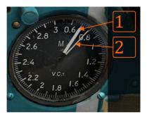
Thick needle (1) shows the M number starting from 0,6 M. Thin needle (2) shows the TAS starting from 600 km/h (on 0,6 mark). Scale indication follows this logic.
