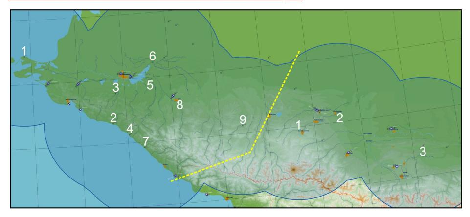
Image 9.5: Ground radio stations locations and ARC channels for sectors 2-I (left) and 2-II (right), divided by yellow dotted line. Outlined in blue lines is radio stations signals coverage area in this sector. This image is available for hi-resolution print (Mods\aircraft\MiG-21BIS\Doc\Manual\_Images).
