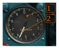
The IAS indicator (US-1600) shows Indicated Airspeed up to 1600 km/h. It has one needle (2) and one window (1). This window will show "1" when IAS is >1000 km/h.
