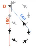
D) Finally, imagine that you are flying on a radial 180 on a southern heading, while you have selected radial 140 and you want to fly towards the station (3K needle points to 320). The director will give you a left turn instruction, constantly giving you leftwards corrections. Apply the same logic as before, allowing for an error of 1/4-1/3 needle deflection before you start adjusting the position according to localizer needles.
