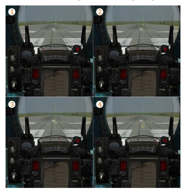
**Image 10.5**: Illustration of the relation between the distance (introduced with throttle rotator) and pipper size and intercept angle.
