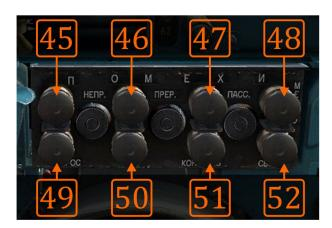
Image 10.8: Radar countermeasures and auxiliary control panel.
