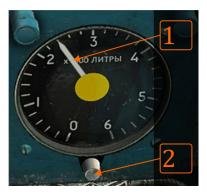
The Fuel quantity indicator shows overall remaining fuel state in liters Knob (2) serves to set initial fuel quantity (pre-flight setup). If the fuel delivery system fails, e.g. fuel from wing tanks is not being used for some reason, indicated fuel quantity will be higher than the actual amunt available. Therefore,
