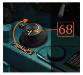
All cockpit light controls are located on the right side panels. There are four knobs for cockpit illumination control. With knobs RH46 and RH48 you control the front panel instruments illumination (48) and text illumination (46). Knob RV5 controls white light that illuminates right vertical panel: this light is used during the start-up procedure. White
