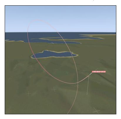
**Image 8.4**: Profile of an inclined loop, left in this case. Speed in inclined loop is better preserved than in a loop, so energy levels are higher. Inclined loops (or their parts) are very useful during combat maneuvering.
