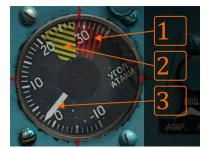
The UUA-1 shows current AoA (3). Readings are precise if IAS>100 km/h and flaps are retracted. If flaps are extended, readings are 2-3° smaller than the actual AoA. The yellow-black sector (2) indicates the best performance zone (maneuverability considering AoA) while the red-black sector (1) indicates the danger AoA zone (critical AoA is 33°, which - if exceeded - will cause a stall, possibly followed by spin). A pilot can safely perform maneuvers up to 28°
