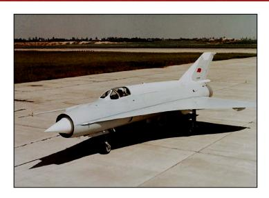
1961: MiG-21I "Analog", test-bed for research and development of Tu-144 passenger airplane wing
