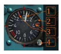
The Accelerometer shows current (1) and maximum/minimum gload (3) achieved during flight. Maximum and minimum loads can be reset using button (4). This is a very important instrument, especially if the aircraft has external loads and g-load needs to be controlled to avoid the load falling off, possibly damaging the airframe or other planes in formation, or causing damage to civilian infrastructure or people.
