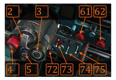
**Image 10.13**: Tactical release switch (CL73) and BOMBS ARMED light (CL72). CL61 and CL62 are payload jettison buttons under the red caps.
