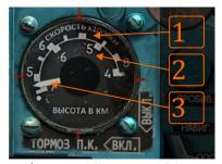
The ARU is a device that controls the ratio between stick pitch and horizontal tail movement. The ARU-3VM gauge shows the current position of the ARU arm transpositioned to a speed-altitude scale. The Speed scale (1) and altitude scale (2) serve to provide a rough orientation whether the ARU system functions as expected. For example, the ARU should be at "long arm" (needle to utmost left, maximum horizontal tail deflection available) if the speed is <=450
