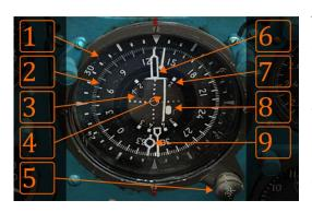
The Course System (NPP) is a complex instrument showing current magnetic heading, direction to a selected NDB or RSBN station (9, pointer at tail), desired course or radial (6, pointer at head, set up with button 5), correct reception of localizer (3, K-"kurs") and glide slope (8, G - "glisada") signals, aircraft position in reference to localizer and glide slope signals (central white needles), relative angles necessary for landing pattern creation (7) and relative
