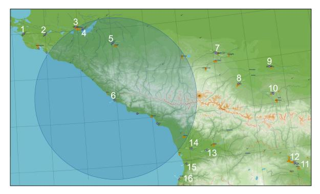
Image 9.8: RSBN/PRMG ground stations at various airports, with channel numbers (1-16). RSBN ground station range/coverage is given for Sochi-Adler only (showing range/coverage for all RSBN's would cover entire image). This image is available for hi-resolution print (Mods\aircraft\MiG-21BIS\Doc\Manual\_Images).
