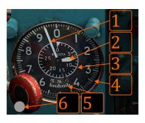
The Barometric altimeter (VDI-30K) measures barometric altitude up to 30km. The small needle (2) points to an altitude in km (scale 3) while the big needle points tens of m (1). The pilot can set the desired atmospheric pressure in window (5) using button (6).
