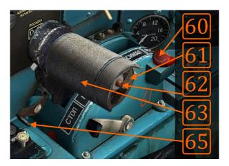
**Image 10.4**: Throttle rotator (LH63): when used with the radar it moves TDC up/down, when used with the ASP it is used to measure the distance to the target.
