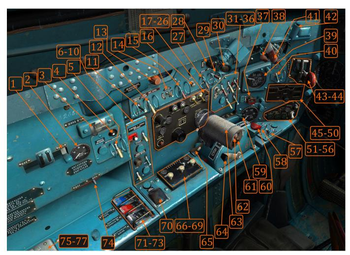
L segment holds the engine management interface along with engine nozzle controls, gears/flaps/brakes controls, the ARU-3VM control panel, RSBN/PRMG control panel, life support system interface, and important emergency engine controls.
