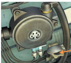
Pressurization control valve (right cockpit side)
