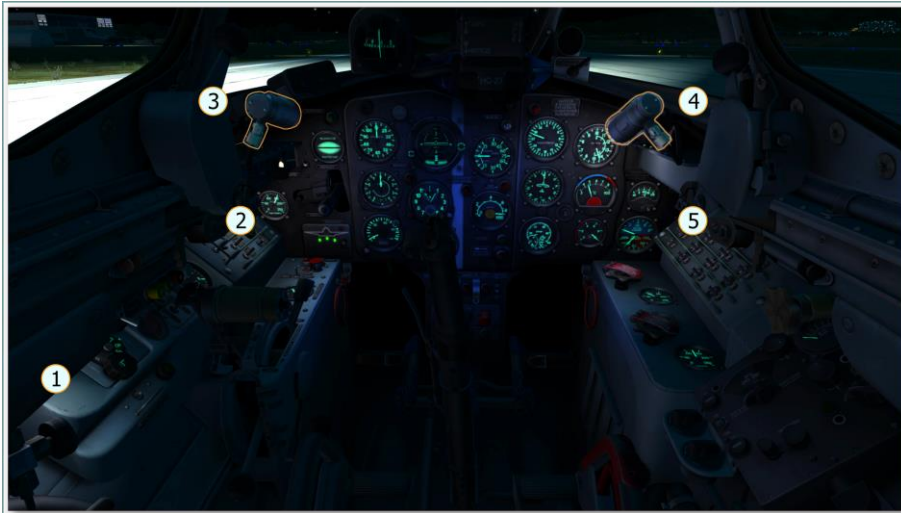
Figure 5.19. Location of MiG-15bis cockpit light sources
