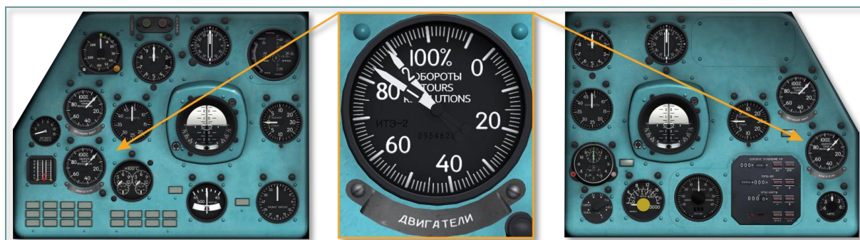
Fig. 5.20. Pilot's and copilot's dual engine tachometers
