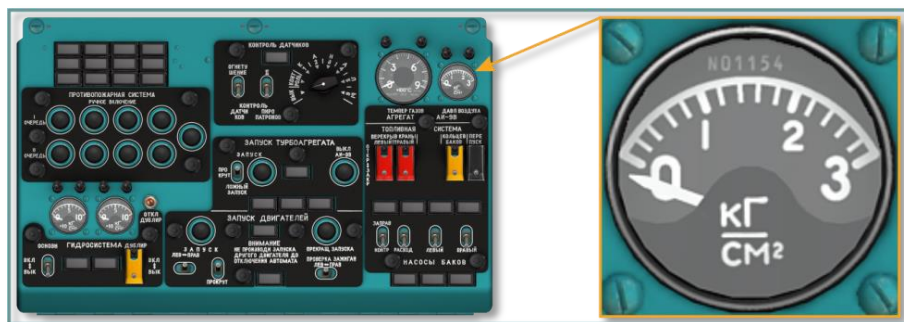
Fig. 5.29. APU air pressure gauge, center overhead console
