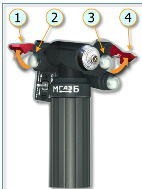
Fig. 7.43. Cargo release buttons on the collective
