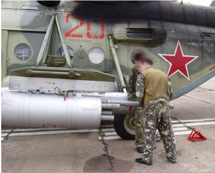
Fig.11.13. Loading of a B8V20-A rocket launcher on an Mi-8MTV5 helicopter.
