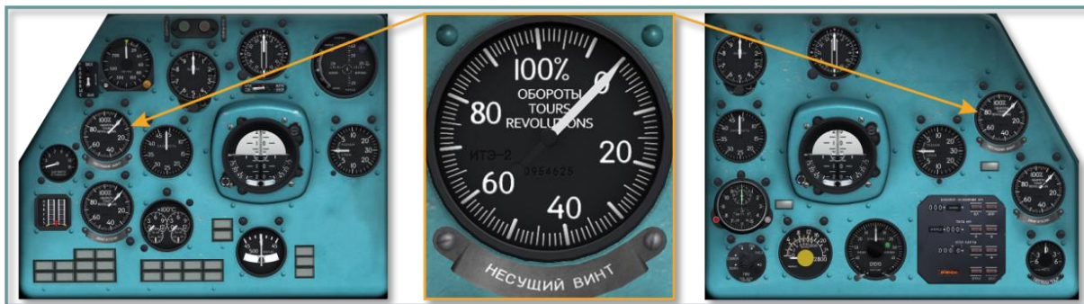
Fig. 5.21. Pilot's and copilot's main rotor tachometers
