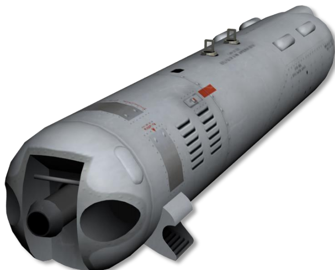
Fig. 11.19. GUV-1 equipped with automatic grenade launcher
