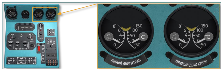
Fig. 5.22. Oil pressure/temperature gauges, center console
