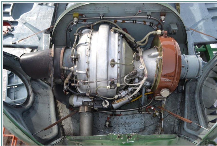
Fig. 4.6. AI-9V APU mounted on the helicopter
