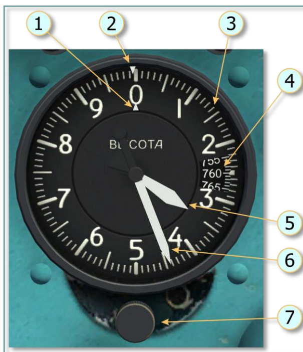
Fig. 5.41. Pressure altimeter function elements
