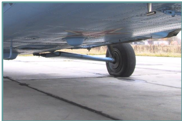
Fig. 6.15. ARK-UD loop antenna housing
