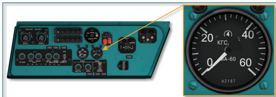
Fig. 5.35. Brake pressure gauge, left side panel
