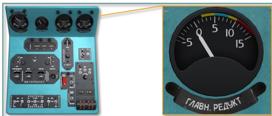
Fig. 5.26. Main transmission oil temp gauge, center console
