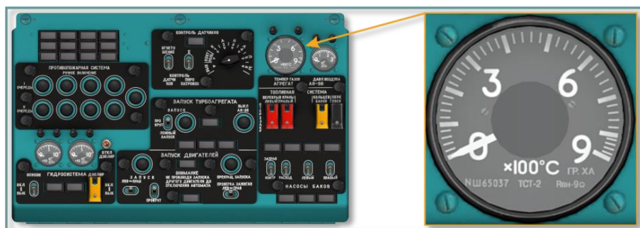
Fig. 5.28. APU EGT gauge, center overhead console
