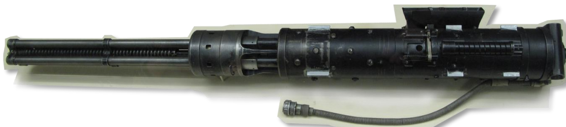
Fig. 11.22. YakB-12.7 12.7 mm 4-barrel Gatling gun
