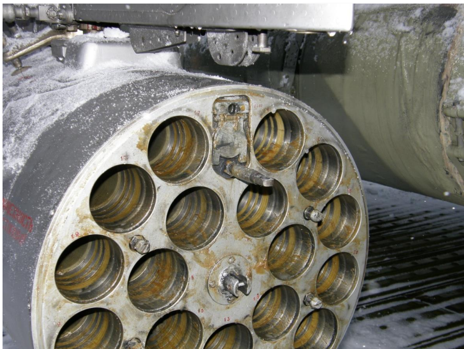
Fig.11.14.B8V20-A launcher tubes as seen from the rear.
