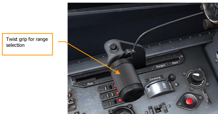
Figure 44: Throttle lever with twist grip and cable
