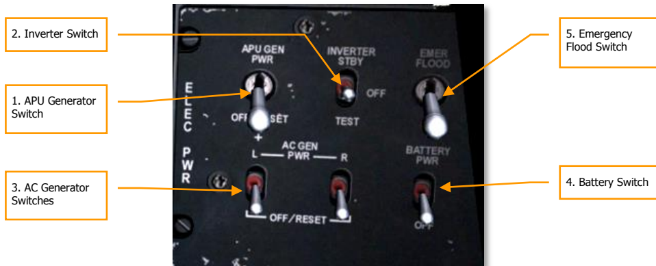
Figure 303. Electrical Power Control Panel
