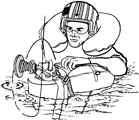
3. SIT ON SEAT FACING FLotation COLLAR. USING ELBOWS, SEPARATE LPA WAIST LOBES AND PULL SHAFT OF PENETRATOR CLOSE TO CHEST.
