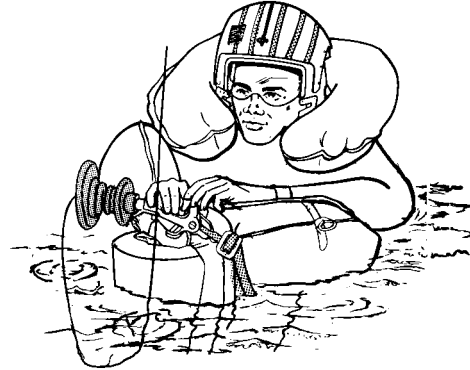
4. PASS SAFETY STRAP UNDER ARM, AROUND BACK, AND UNDER OTHER ARM. CONNECT SAFETY STRAP AND TIGHTEN.
