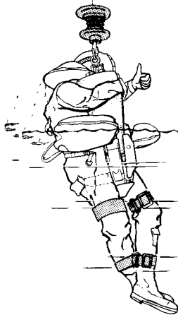
5. TURN HEAD DOWN AND TO THE LEFT. GIVE THUMBS UP SIGNAL TO HELO-HOIST OPERATOR.
